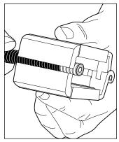
Remove about 1" (25 mm) of the jacket from the cable end by scoring and slicing the jacket.
