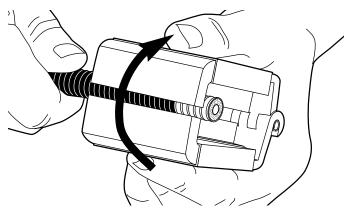
Lightly squeeze the tool halves together and rotate the tool clockwise (as viewed from the cable end) three or four revolutions to score the outer conductor. Then, firmly squeeze and rotate the tool until the cut section falls away. Note: Keep a firm and constant grip on the tool. Do not release the tool during rotation because this will result in an uneven cut. Proceed to the connector installation bulletin.
